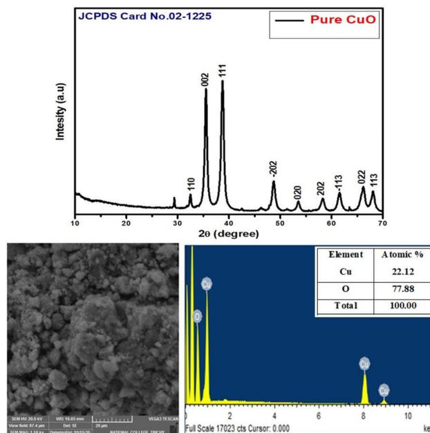
Figure 2: XRD, FESEM and EDAX analysis of chemically synthesised CuO NPs.
