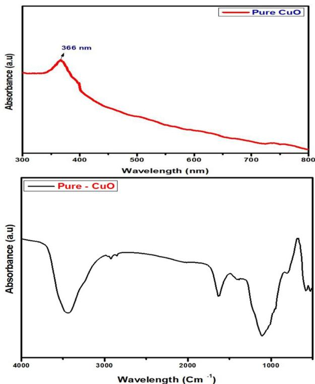
Figure 1: UV and FTIR spectrum of synthesised CuO nanoparticles.
